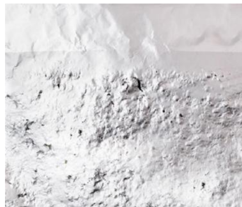
Note the even distribution of perforations in the foil and the line where submersion started
